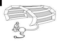
Stack the inflatable on top of itself so that during inflation it will rise vertically.
